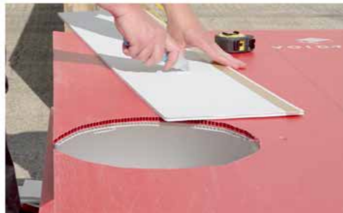
To strengthen and support the front edge, cut one of the spare internal fins to size.
